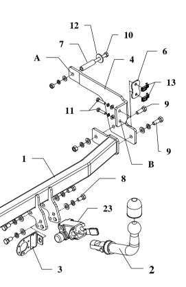
This towbar is designed to assembly in following cars: **RENAULT LAGUNA 5 doors,** produced since 2001 till 2007, catalogue no.**G39A** and is prepared to tow trailers max total weight **1500 kg** and max vertical load **75 kg**.
