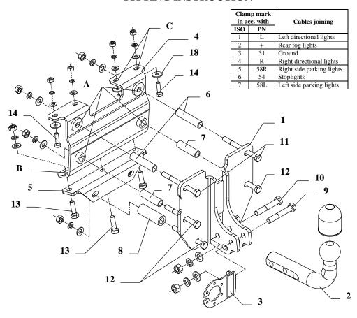
This towbar is designed to assembly in following cars: **OPEL ASTRA F ESTATE,** produced since 09.1991 till 2002, catalogue no. **E36** and is prepared to tow trailers max total weight **1500 kg** and max vertical load **50 kg**.
