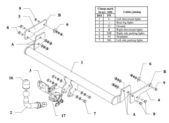
This towbar is designed to assembly in following car: CITROEN ZX 3/5 DOORS, produced since 1991 till 1997, catalogue number P03A, and is prepared to tow trailers max total weight 1100 kg and max vertical load 70 kg.
